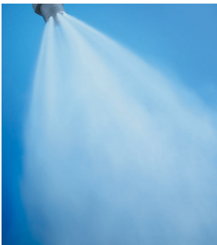
Spray atomisation for gas cooling and conditioning in cement plants
