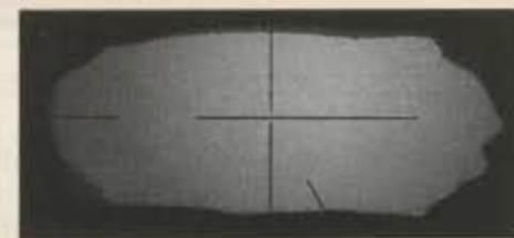
worn spray tip magnified
